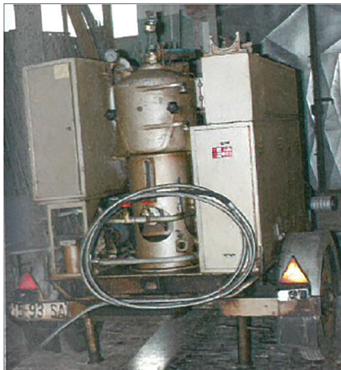
Figure 13.11 Transformer oil filtering machine, GALILEO MODEL 26 A512, in use since the 1960s
