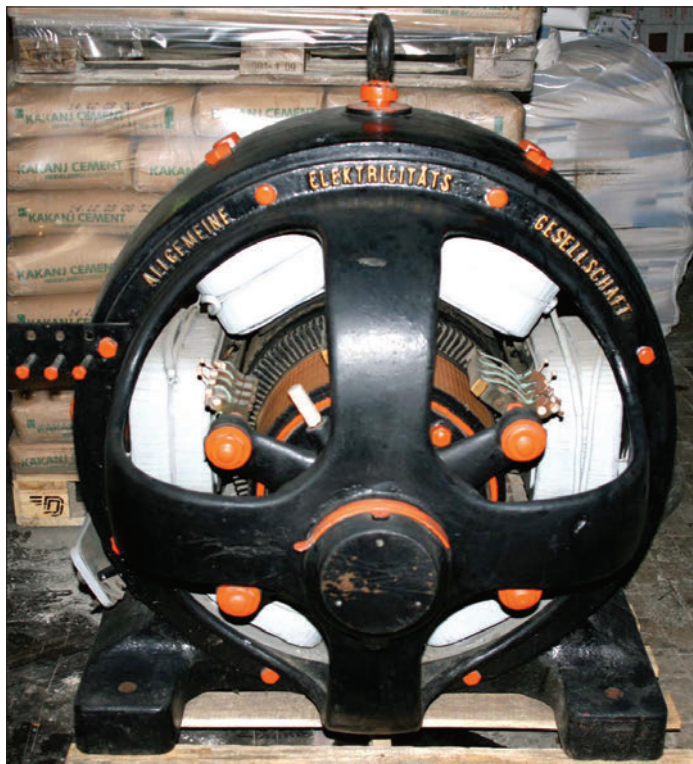
Figure 13.9 Dynamo generator Type EG 650. (AEG production before the First World War)
