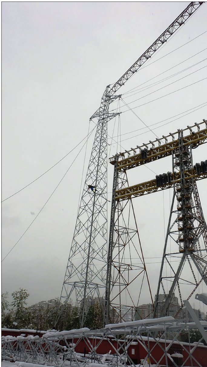
Figure 3.19 Energoinvest's test station for transmission poles, Alipašin Most a) Preparation for the test (left), b) Testing the bearing capacity of the power line pole (right)
