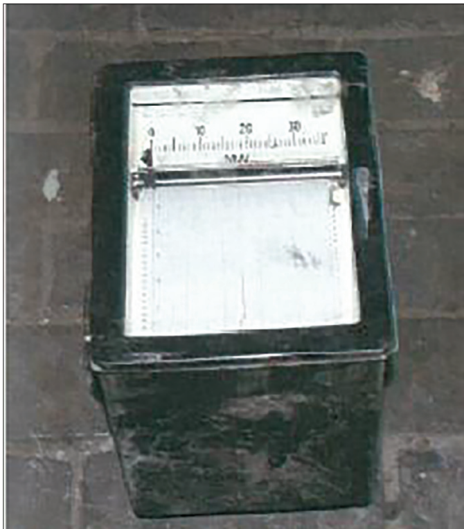
Figure 13.8 Recorder, range 0-36 MW, Manufactured by SIEMENS, 1956
